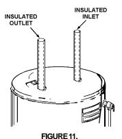
Fit pipe insulation over the incoming cold water line and the hot water line. Make sure that the insulation is against the top cover of the heater. Fit T & P valve insulation over valve. Make sure that the insulation does not interfere with the lever of the T & P valve.
